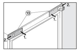
■ Click covers ③ into place on both sides from the front. Guide the cover with the cut-out over the bearing block.
